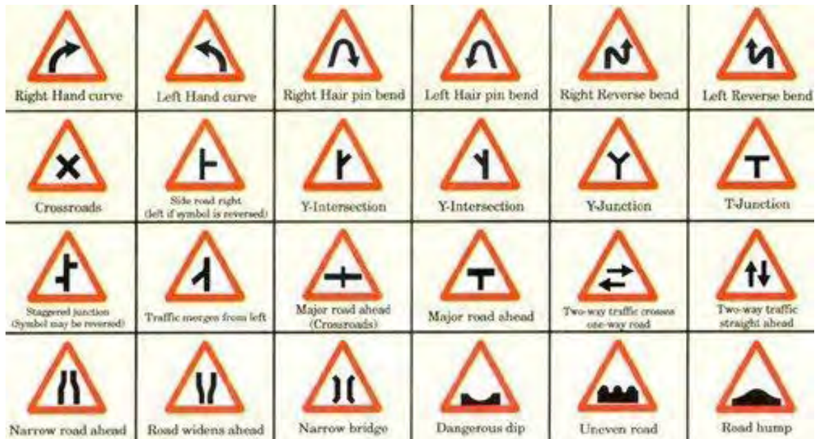
FIGURE 6-61 Cautionary or Warning Signs
