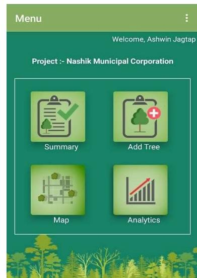
The home screen of the application consist of 4 main options namely Summary, Add a tree, Map and Analytics. Before, the field officer fill in the survey form, the device checks the accuracy and thereafter allows the surveyor to conduct the activity.
