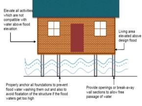
Figure 10.5 : Structures Allowing Free Water Flow from Below
