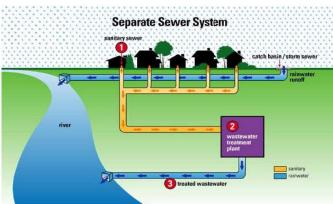
Figure 10.8 : Separate Sewer and Storm
