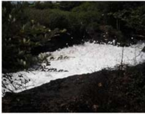
Excessive foam formation in treated effluent from Tapovan STP
