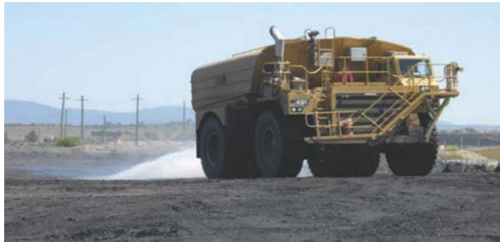
Figure 1 : Road side sprinkling of dust control agents
